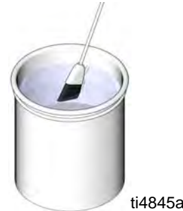
Fig. 14: Use solvent-dipped soft-bristle brush
