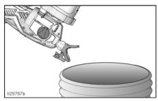
8. Turn Prime Knob forward to SPRAY position. Rotate Spray Tip 180 degrees to UNCLOG position.
