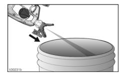
Reverse the Spray Tip to UNCLOG position, pull the Trigger for 30 seconds until sprayer is clean.
