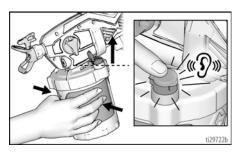
**NOTE:** If FlexLiner is not squeezed while VacuValve Cap is open, air will quickly pull into the FlexLiner. If any air bubbles are visible in the cup, repeat steps E-G.
