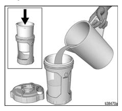
3. Firmly tighten Cup Lid onto the Cup Support to ensure an airtight seal.
