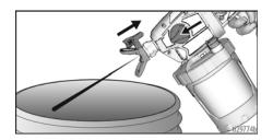
Turn Prime Knob downward to PRIME position. Rotate Spray Tip back to SPRAY position. Turn Prime Knob forward to SPRAY position, and resume spraying.
