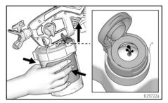
g. While continuing to squeeze the FlexLiner, close the VacuValve cap.
