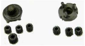
7. Disassemble the planetary gears and the pinion gear from the spindle assembles. Inspect the gear teeth and shaft holes for wear and damage. A pinion gear is used on the 4 Nm and 8 Nm tools only.
