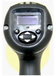
2. Using a T-10 Torx Bit remove the two display panel screws.
