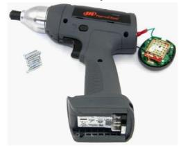
20. Gently lower the housing down onto the unit. Ensuring that all of the components and cables are in their proper position. Closing the tool by starting at the bottom at the foot PCB and working your way to the motor and the top of the tool.
