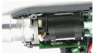
14. Connect the Hall Cable with its connector on the motor.
