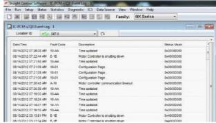
Select QX Series under family then under the Run tab in the main menu bar, click on and run the IC-PCM/QX Event Log and select Location
