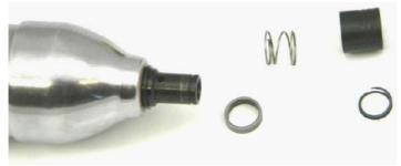
1. For units with the \%"quick change spindle, disassemble the spindle as follows. Remove the spiral spring clip from the front of the spindle, then remove the quick change collar, spring, spring support and rear spiral snap ring.
