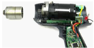
9. If the Gear Pack has remained on the motor, remove it from the motor, and set aside. We will disassemble this later in the program.
