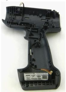
5. Route the hall cable through the housing following the shadow line, leaving approximately 1 ½" of cable above the housing where the cable connects to the motor.
