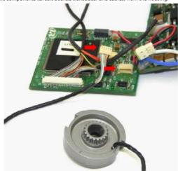
14. Disconnect the transducer cable from the Foot Control Board.
