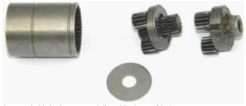
$5. \ \ \, \text{To disassemble the gear pack, slide the planetary gear spindles and the plate out of the ring gear.}$
