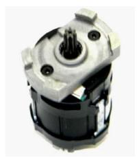
1. Install the motor mount onto the motor. Align the mount so that the slot in the mount is on the opposite side of the motor from the motor connector as shown in the photo. Torque the motor mount screws to .5 Nm.
