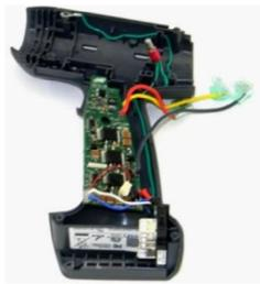
6. Route the green ground wire through the housing and to the top front screw lug.
