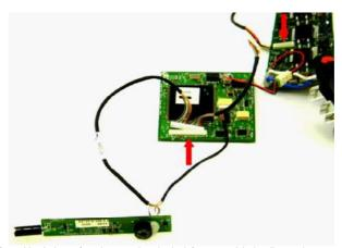
15. Disconnect the Interface cable which runs from the trigger board to both foot PCB and the handle PCB. There is one connector on the foot PCB and one on the handle PCB.
