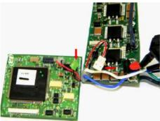
17. Disconnect the Handle PCB from the Foot PCB at its connector. This completes the disassembly of the electronic components.
