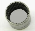
6. Inspect the ring gear for wear and damage.
