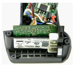
12. Install the foot PCB and the battery interface. Retrace and fully seat all the cables, ensuring that they are in their proper position. Also ensure that the trigger board is still in place. Any cables which are not seated properly will be damaged resulting in the tool not performing properly.
