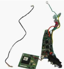
16. This will leave the Hall Cable which can now be disconnected from the foot board and the cable removed.
