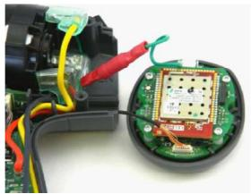
18. Connect the ground cable connector and the Interface cable connector to the display board.
