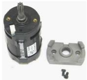
12. Using a 2mm Allen wrench, remove the two Allen Screws which hold the motor mount onto the motor. Then remove the mount.
