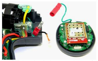
5. Disconnect the pin connector first, then disconnect the ground wire slip connector. Remove the USB port cover from its slot in the housing.
