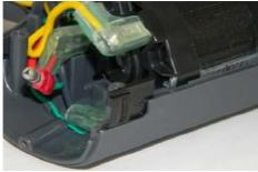
17. Install the USB port cover into its slot.
